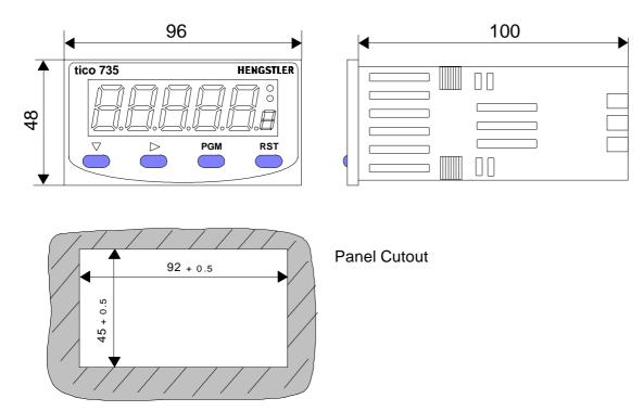
Insert the unit in the panel through the cutout. Ensure that the panel gasket is not distorted and the instrument is positioned squarely against the panel. Slide the mounting clamp into place on the instrument and push it forward until it is firmly in contact with the rear face of the mounting panel and the tabs on the bracket arm are seated in the mounting grooves on the side of the unit.
